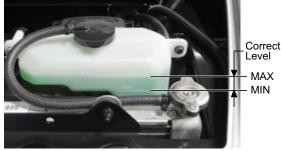
NOTICE: If coolant runs low often, or if the coolant reservoir runs completely dry, check for leaks within the cooling system.
